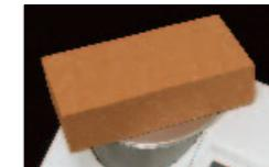
By using the Ø3 mm target mask (optional accessory), even small samples can be measured.
