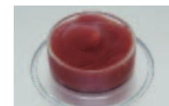
Colorant pellets can be measured in raw form using a Petri dish (optional accessory).
